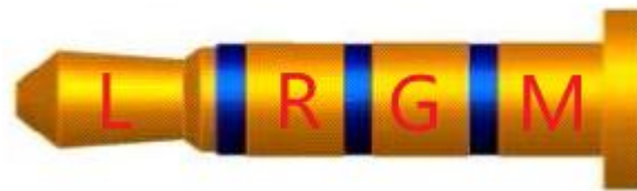
Figure 15 Definition of four-segment headphones
